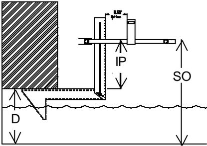
**Measure from top inside of pipe to top of frame then add pipe diameter to get sensor offset or measure from the top of the frame to the bottom of the pipe.**
